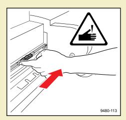
4 Remove the jammed media. For all types of media jams, always inspect the drum and rollers for any loose paper and remove it.
